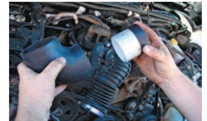
30. Loosen the factory air intake hose at the throttlebody and turn the hose counterclockwise, facing down toward the new intake location. Use the second supplied 90-degree elbow, the aluminum connector with the rubber spacer (the end of the tube with the spacer connects to the throttlebody hose) and the hose clamps to assemble the throttlebody intake components. Make sure all of your connections are sealed tight.
