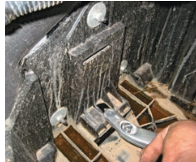
15. At the rear of the factory battery tray there are four plastic gussets that must be removed. You can do this with a utility knife.
