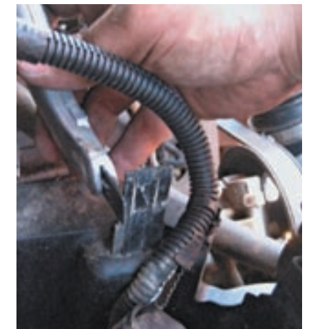
21. With a utility knife, shave both sides of the mounting post to allow the unit to slide further down.
