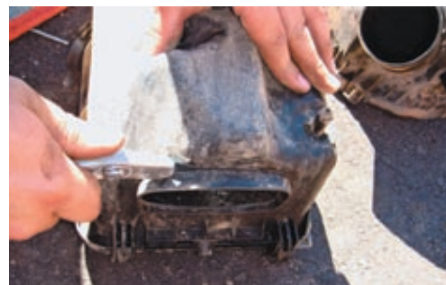
3. This plastic lip on the air box needs to be trimmed flush with the air box surface as shown. Using a utility knife, trim the plastic lip on the old intake location so that the new block-off plate will sit tight against the air box.
