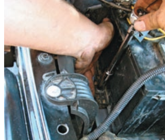
(Left) 28. Reinstall the battery in its new location, making sure to secure it with the factory hold-down. Once the battery is secured, slide one end of the supplied rubber intake hose over the end of the aluminum snorkel tube until it is tight against the fender, then secure it with the supplied hose clamp. Route the new intake hose along the battery, turn and go over top of the unit that you lowered, then over to the top of the factory air box.
