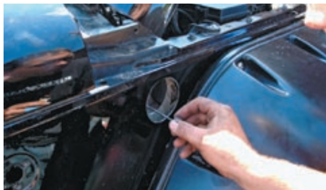
25. Remember to paint all bare metal to keep rust from forming.
