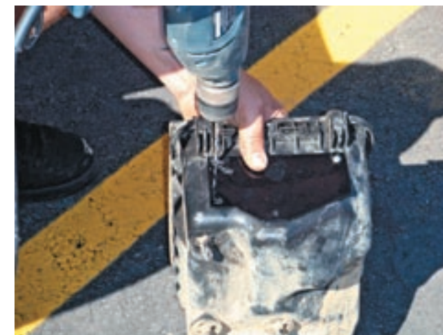
4. Take the supplied block-off plate and position it over the factory intake hole, then drill the four mounting holes.
