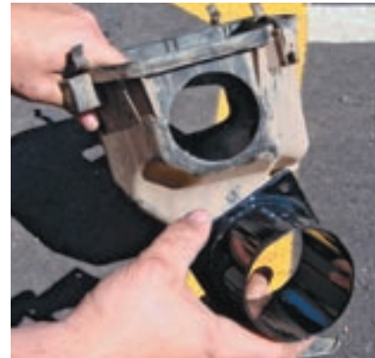
11. Test fit the new intake bracket. Once it fits, drill the four mounting holes.
