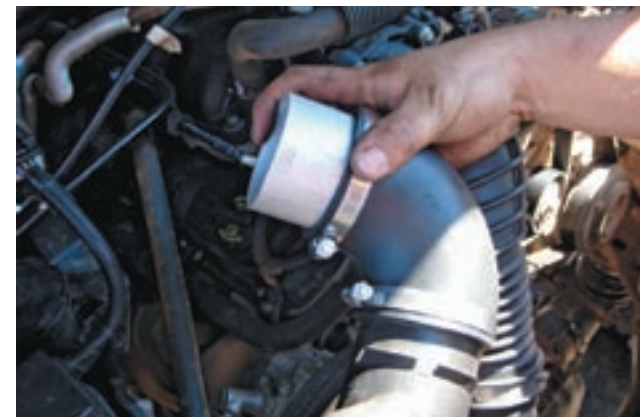
29. Use one of the aluminum connectors, the supplied 90-degree elbow and the stainless steel hose clamps to connect the intake hose to the top of the air box.
