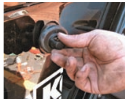
14. For ease of installation we recommend that you carefully remove the passenger-side front fender flare. If, however, you have a second set of hands available, it can be done without removal. The antenna and the battery must be removed to continue. For the proper installation of this system, the battery location must be adjusted.
