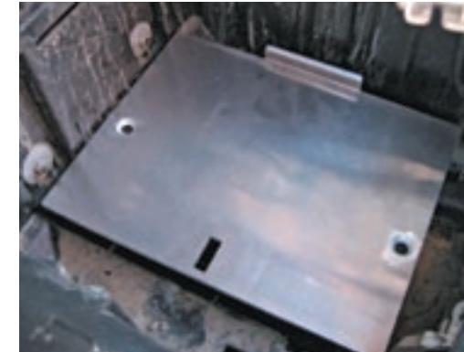
(Right) 17. The new battery tray is secured with supplied stainless steel bolts, lock washers and nuts. Position the aluminum battery tray with the bent tab upright, facing toward the engine. Leave approximately 3/8-inch between the plastic shield (that is between the engine and the battery) and the new battery tray. Now drill the mounting holes down through the battery tray and into the plastic below, and attach with the supplied hardware.
