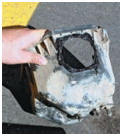
12. Again, apply a healthy bead of 100 percent silicone to ensure a watertight seal between the air box and the intake bracket, then attach the bracket with the supplied stainless steel hardware.
