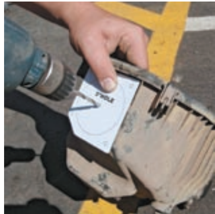
9. Now take the supplied template marked "JK AIR BOX" and position it on the air box. This will show you where to drill the three-inch hole for the new intake.
