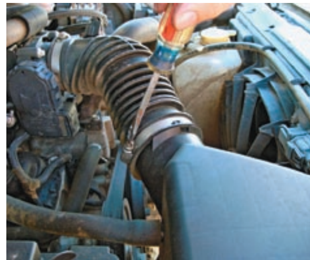
1. Remove the factory air box. Disconnect the throttlebody hose, the breather hose and unbolt the box.
