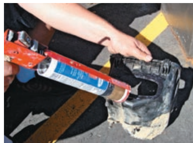
5. Apply a healthy bead of 100 percent silicone around the block-off plate mating surface to ensure a watertight seal between the plate and the air box.
