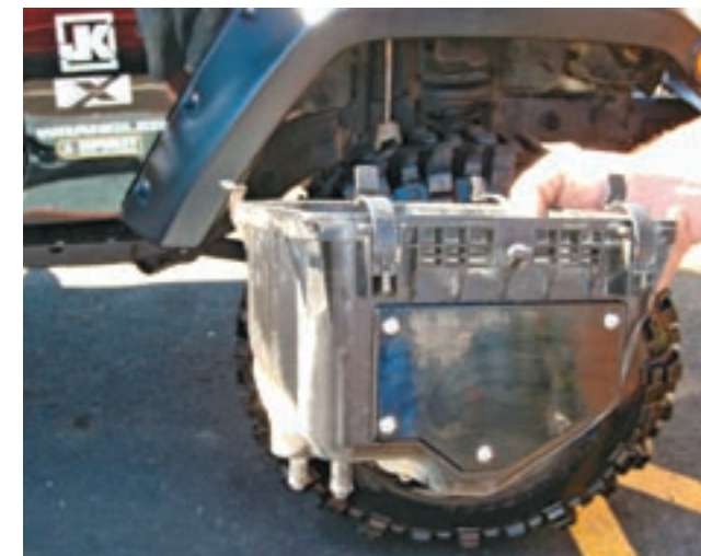
6. When the silicone has “skinned over,” attach it to the air box with the supplied stainless steel hardware.
