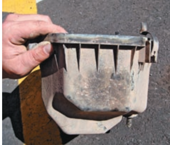
7. The new intake location will be positioned on the other side of the air box.
