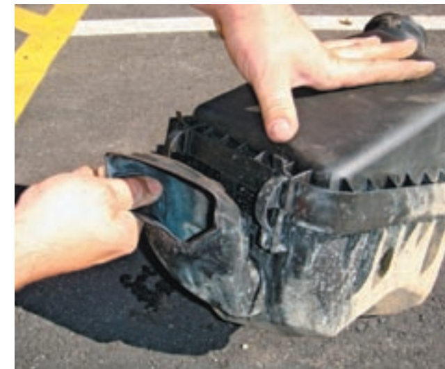
2. Remove the intake tube from the factory air box.
