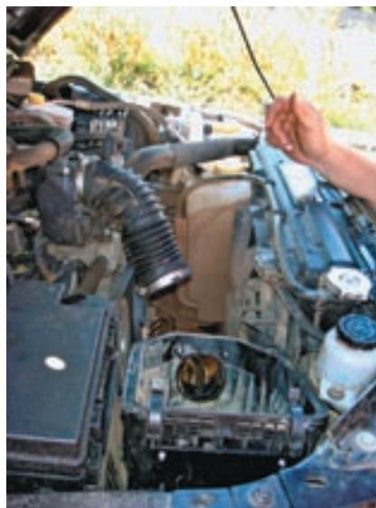
13. Reinstall the air box in the engine compartment.
