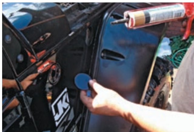
27. A supplied aluminum block-off plate is included to cover the factory antenna location. It can be painted to match your vehicle and siliconed in place.
