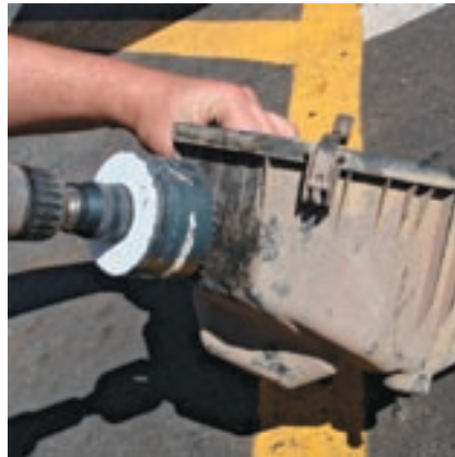
10. Now drill the three-inch hole in the side of the air box.
