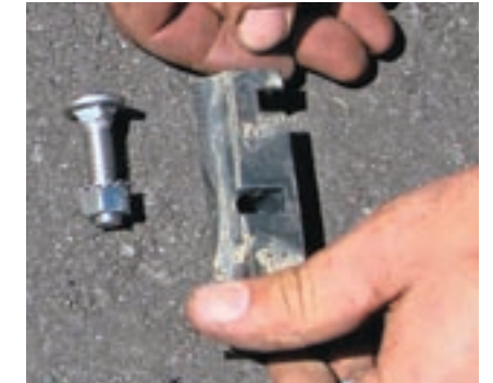
18. The factory battery hold-down is re-used, however, it must be drilled out to accept the supplied 3/8-inch carriage bolt and hardware.
