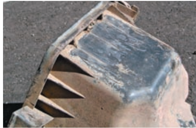
8. Trim the three plastic ribs on the side of the air box so that they are flush with the box surface.
