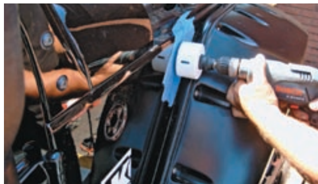
24. Using a three-inch hole saw, drill the hole in the fender. You will be cutting through several layers of metal, so be sure you drill at a 90-degree angle to the surface of the fender to ensure that the snorkel will fit properly.
