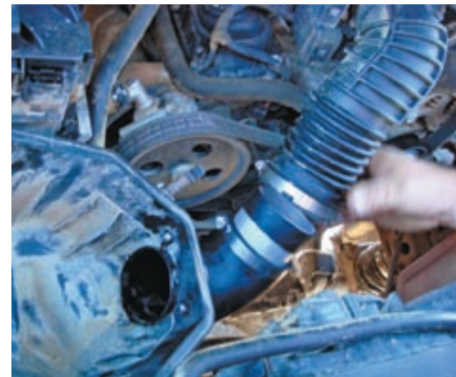
31. Attach this assembly to the throttlebody intake tube and to the air box as shown.
