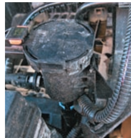
19. Now turn your attention to this small unit positioned next to the battery tray that has several black airlines attached to it. We are going to lower it approximately one inch. Begin by sliding it off of its mounting post.
