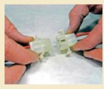
The connector then snaps together and can be disconnected whenever you need to remove your transceiver from your Jeep.
