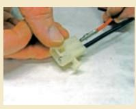
The supplied male pins are secured to one side of the circuit while the female pins are secured to the other side. The pins are then inserted into the plastic plug (male) or receptacle (female). The only trick is to make sure that the power and ground wires correspond to each other on each side of the connector.
