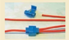
The quick-splice connector is the best way to tap one wire into another, such as when tapping into a power lead. One side of the connector fits over the main wire while the add-on wire fits into the other side (which is blocked off at one end). Once in place, you can use a pair of pliers to push the metal connector bridge over the wires (which cuts into the insulation to make the electrical connection). Lock the security tab in place to finish.
