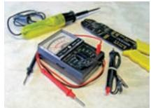
It doesn't require a lot of expensive or fancy tools to work basic automotive electrical systems. The key ingredients are a quality wire stripper/crimper tool (one that denotes wire gauge for stripping insulation and crimping connectors), followed by a test light or two and a decent multimeter—preferably one capable of measuring DC voltage, DC amperage, milliamps and ohms
