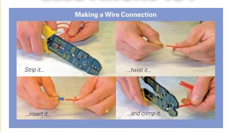
some situations when you are connecting directly to the battery positive terminal. A bare wire exposes your electrical circuit to shorts, which can damage fragile electrical components or, worse yet, cause a fire.
